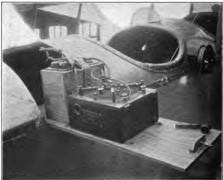
Plate 12. —An induction coil type of spark set operated from the storage battery at the left. Designed and used extensively by the British in airplane fire control work. The antenna tuning inductance is the flat spiral coil mounted on top of the set box. The set and battery are fastened on a sliding shelf for quick removal from the fuselage. Note the antenna reel at the right, outside the cockpit. Present practice is to put the reel inside the fuselage. British Sterling set. Signal Corps set type SCR-65.
